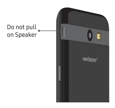
**Warning**: Do not bend or twist the back cover excessively. Using excessive force on the cover during removal or installation of an internal component can cause the material to break.
