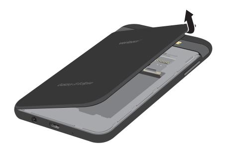
**Caution**: When removing the back cover, use the slot next to the Volume key to gently lift the cover off. Pulling on the Speaker (located next to the Power button) may cause damage.
