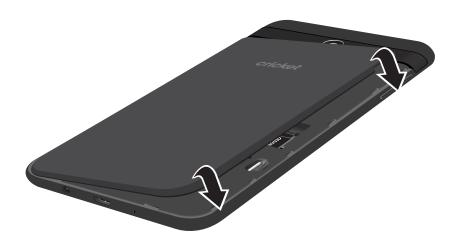
2. Press along the edge of the back cover until you have a secure seal.
