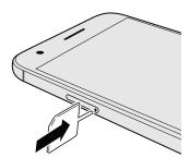
3. Push the tip all the way into the hole until the tray ejects, and then pull the tray out.
