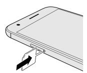
3. Push the tip all the way into the hole until the tray ejects, and then pull the tray out.
