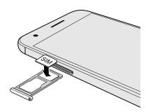
Place your microSD $^{\text{TM}}$  card into the SD holder of the tray. See Inserting the microSD card on page 20.
