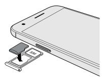
5. When reinserting the tray, make sure it is facing up so that the nano SIM and microSD cards don't fall out. Gently slide the tray all the way into the slot.
