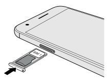
**6.** Press on the cover that's attached to the tray to close it tightly.
