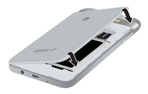
2. Press along the edge of the back cover until you have a secure seal.
