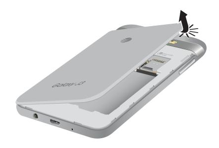
2. Lift the cover up and to the left of the device.
