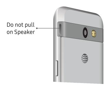
**Warning**: Do not bend or twist the back cover excessively. Using excessive force on the cover during removal or installation of an internal component can cause the material to break.
