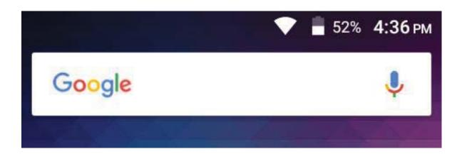
On the notification bar, several icons will appear such as signal bar, battery indicator, data indicator, Bluetooth and Wi-Fi. You may slide the notification bar down with your finger to display any pending notifications or actions.
