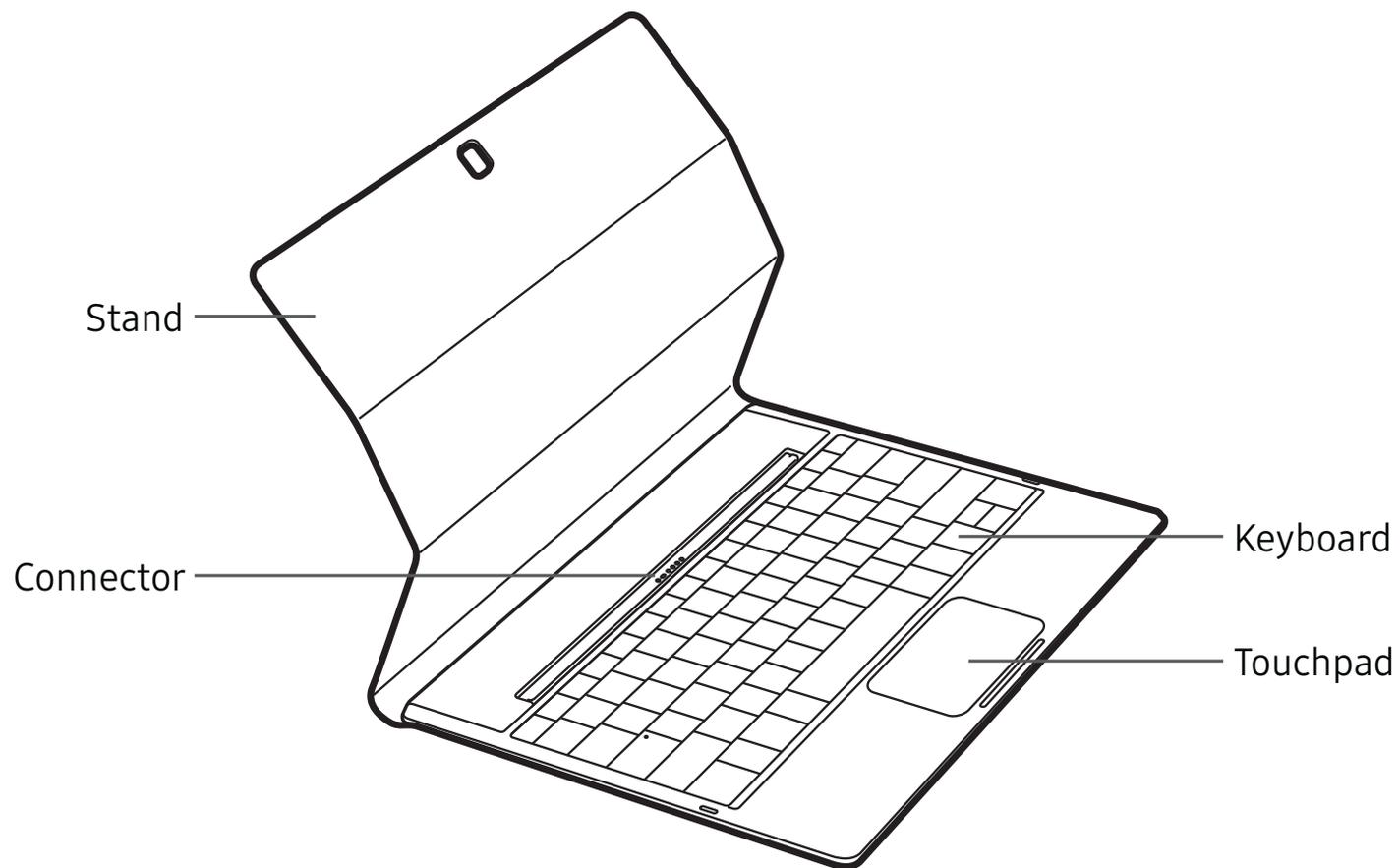
Connecting the device to the Keyboard cover allows you to use a traditional keyboard and touchpad. The touchpad will register pressure on the right or left side, so you can use the touchpad like a mouse. You can also stand your device upright using the stand on the Keyboard cover.
