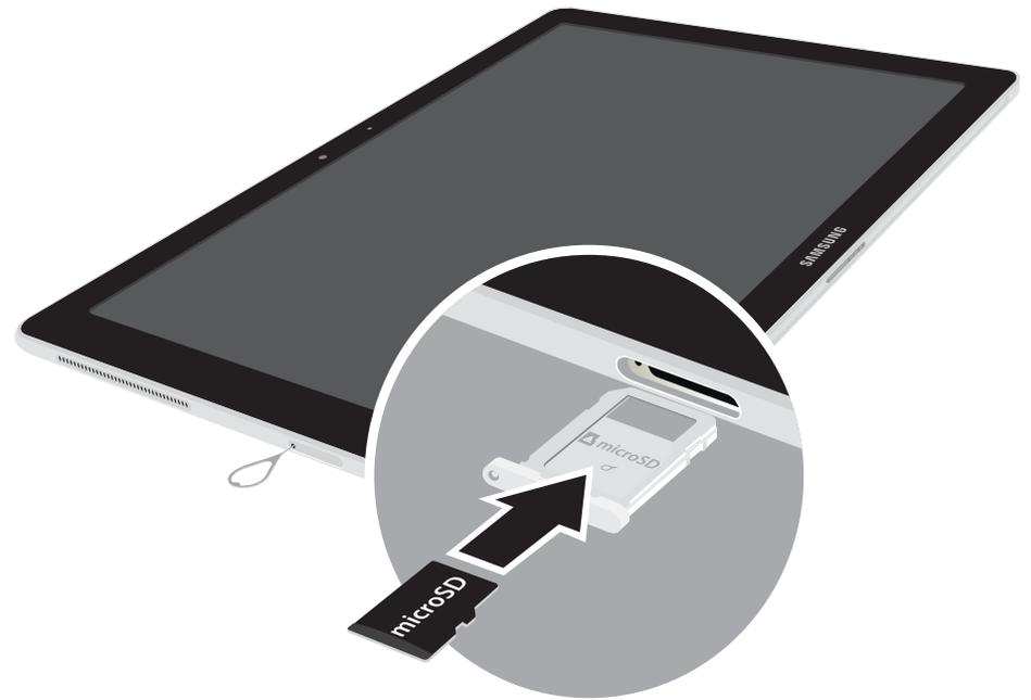
2. Insert the new microSD card into the microSD card tray with the gold contacts facing down.
