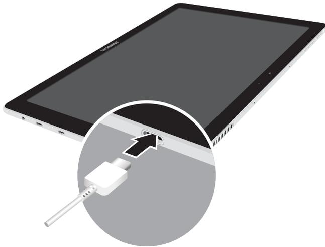
2. Connect the USB cable to the charging head, and then plug the charging head into a standard outlet.
