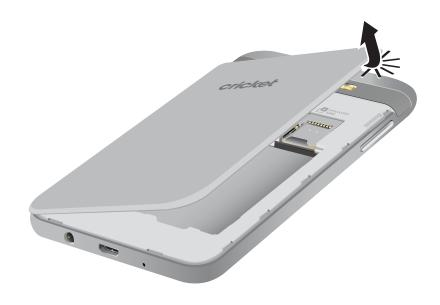
2. Lift the cover up and to the left of the device.
