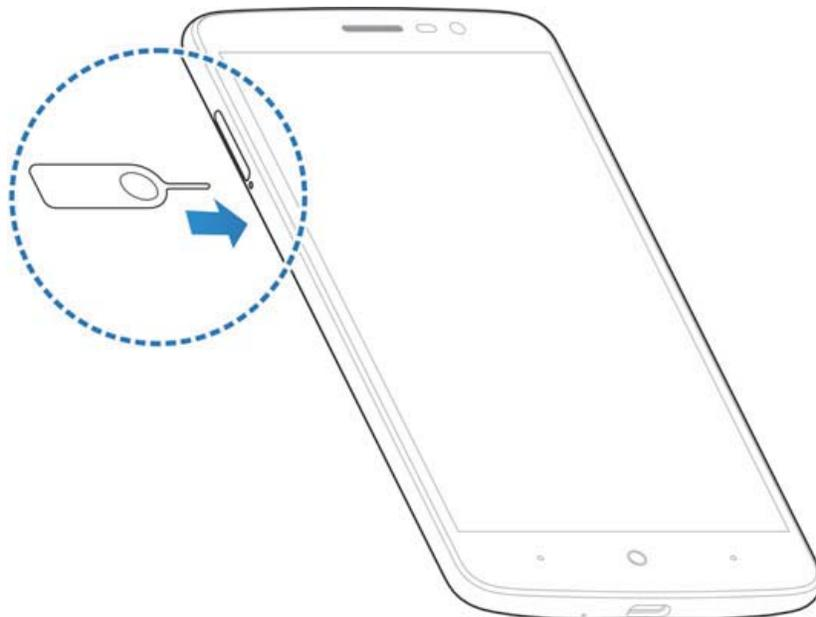
2. Pull out the card tray and place the nano-UIM/microSDXC card (not included) on the tray with the gold-colored contacts facing down. Carefully slide the tray back into place.
