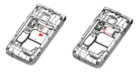
4. Insert the battery. Align the contacts of the battery with the contacts in the phone.
