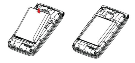
5. Attach the battery cover. Make sure all the table are secure and there are no gaps around the cover.
