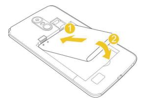
Align the contacts of the battery with the contacts in the phone.
