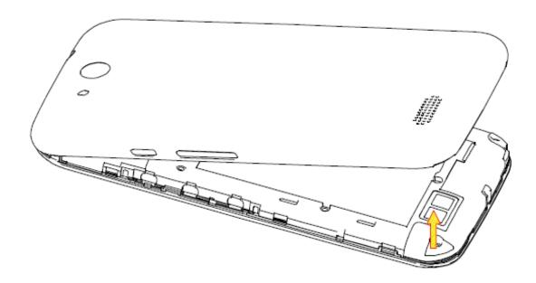
2. Hold the micro-SIM card with the cut corner oriented as shown and slip it into the card holder until you hear a click.
