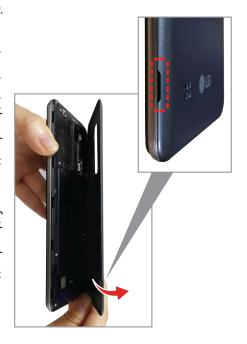
2. Use the fingertip cutout at the bottom of the battery compartment to lift the battery out.
