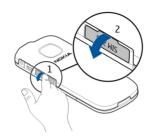
2 Make sure the contact area of the SIM card is facing down, and insert the card (3). Push the card in, until it locks into place. Close the cover (4).
