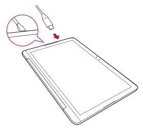
The Charger/USB port (C-type) is located at the bottom of the device. Insert the charger and plug it into a power outlet.
