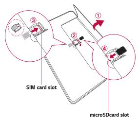
4 If you want to use a memory card, insert the memory card into the slot. Make sure the gold contact area is facing downward. Slide the microSD card into the slot until it "clicks" into place and then close the slot cover.
