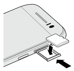
Insert the microSD card tray back into the slot.
