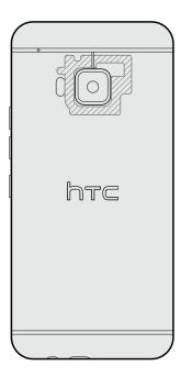
Make sure that the NFC area (shaded part) of HTC One S9 and the other phone's NFC area are close to one another. Experiment by slightly moving the phones until a connection is made.
