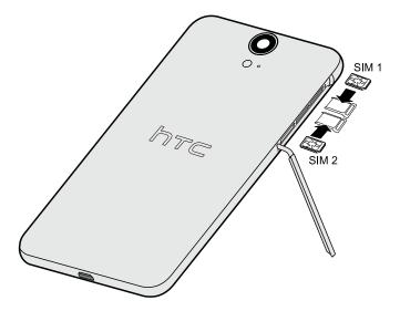
5. When reinserting the trays, make sure they are facing up so that the nano SIM cards don't fall out. Slide the trays all the way into the slots.
