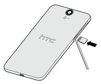
**3.** To close the slot cover, slightly move it side to side to let the rubber hinge sink down by itself. Then gently press down the cover.
