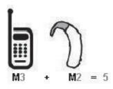
In the above example, if a hearing aid meets the M2 level rating and the wireless phone meets the M3 level rating, the sum of the two values equal M5. This should provide the hearing aid user with "normal usage" while using their hearing aid with the particular wireless phone. "Normal usage" in this context is defined as a signal quality that's acceptable for normal operation.
