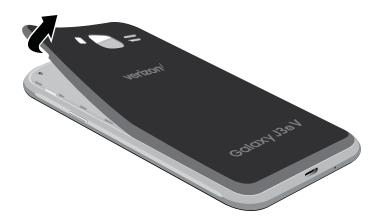
2. Lift the cover up and to the right of the device.
