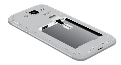
**Caution**: If the SIM card is not inserted correctly, the device cannot detect it. Reorient the SIM card and place it back into the slot if it is not detected.
