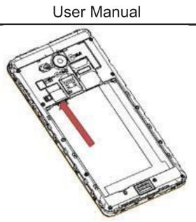
Finally insert the battery and the rear cover of the mobile phone.
