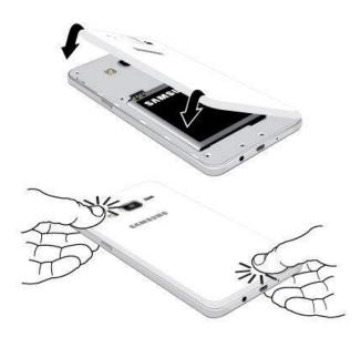
Warning: Do not bend or twist the back cover excessively. Doing so may damage the cover.
