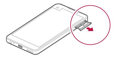
3 Put the SIM card on the card tray with the gold-coloured contacts facing downwards.
