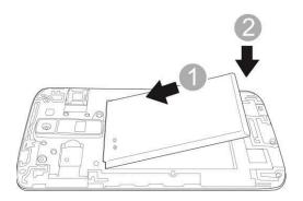
• Align the contacts of the battery with the contacts in the phone.
