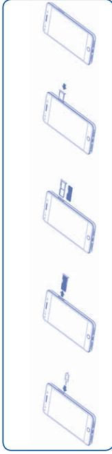
Before you install or remove the SIM card, use a pin to press the small cavity until the SIM cassette pops out.
