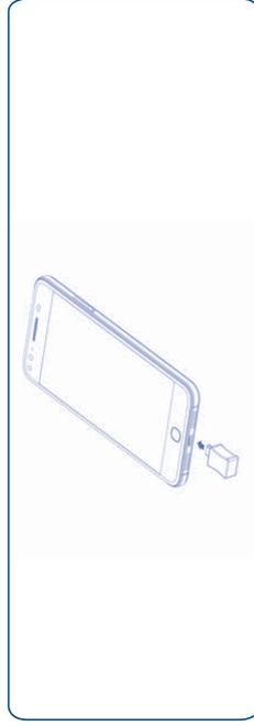
Connect the battery charger to your phone and wall socket respectively, the LED indicator will light while charging.
