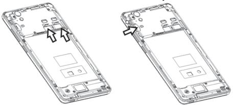
3. Finally insert the battery and replace the rear cover of the mobile phone.
