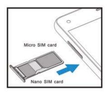
SIM Slot 1: Micro SIM card slot
