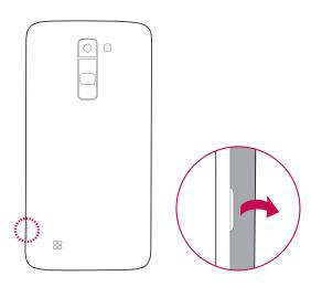
**2** Slide the Nano SIM card into the Nano SIM card slot as shown in the figure. Make sure the gold contact area on the card is facing downward.
