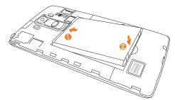
4 To replace the cover onto the device, align the back cover on and press it down until it clicks into place o.
