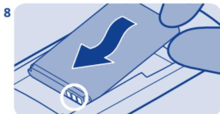
Line up the battery contacts, and push the battery in.
