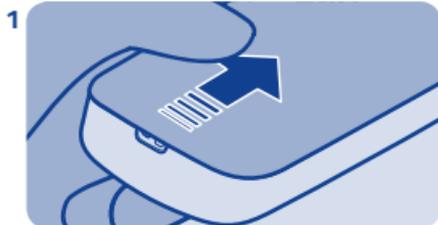
Switch the phone off, then remove the back cover.
