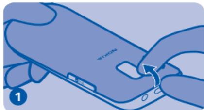
Switch the phone off, then remove the back cover.
