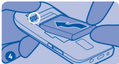
Line up the battery contacts, then push the battery in.
