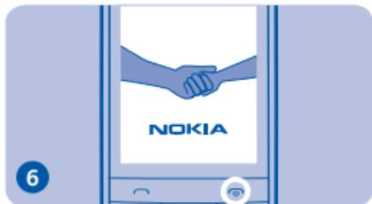
To switch on, press and hold
