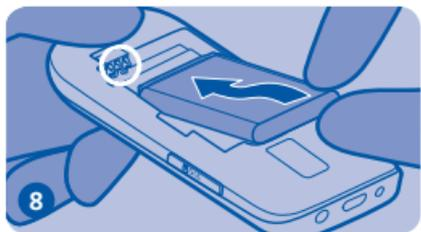
8 Line up the battery contacts, then push the battery in.
