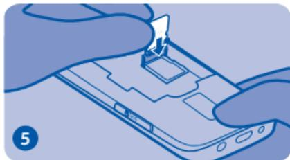
Put a compatible memory card in with the contact area face down.
