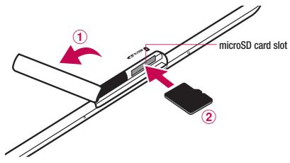
2 Insert the memory card into the microSD card slot. Make sure the gold contact area is facing downward. Slide the microSD card into the slot until it "clicks" into place and then close the slot cover.
