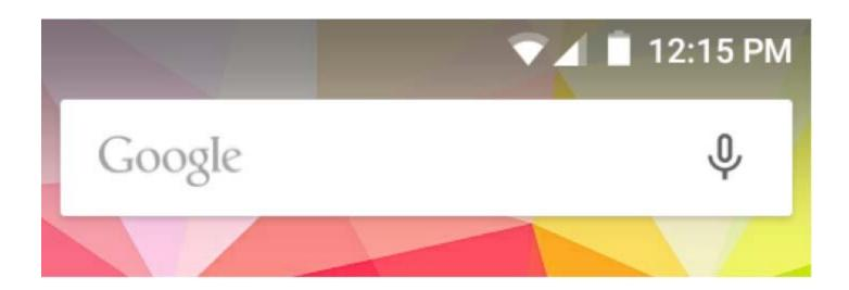
On the notification bar, several icons will appear such as signal bar, time, battery indicator, data indicator, Bluetooth and Wi-Fi. You may slide the notification bar down with your finger to display any pending notifications or actions.
