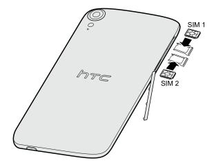
5. When reinserting the trays, make sure they are facing up so that the nano UIM and nano SIM cards don't fall out. Slide the trays all the way into the slots.
