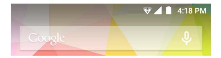
On the notification bar, several icons will appear such as signal bar, time, battery indicator, data indicator, Bluetooth and Wi-Fi. You may slide the notification bar down with your finger to display any pending notifications or actions.
