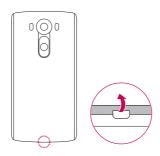
2 Slide the Nano SIM card into the Nano SIM card slot as shown in the figure. Make sure the gold contact area on the card is facing downward.
