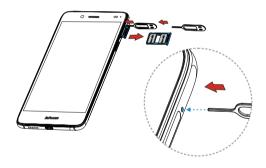
2. Put the SIM1 into the card slot on the tray left side, and put the SIM2 or TF card into the card slot on the tray right side. Then push the tray into the phone card slot.
