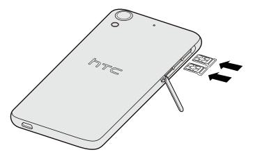
6. To close the slot cover, slide the plastic hinge into the side and press the cover until it clicks into place.
