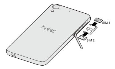
5. When reinserting the trays, make sure they are facing up so that the nano SIM cards don't fall out. Slide the trays all the way into the slots.
