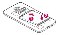
4 To replace the cover onto the device, align the back cover over the battery compartment 1 and press it down until it clicks into place 2.
