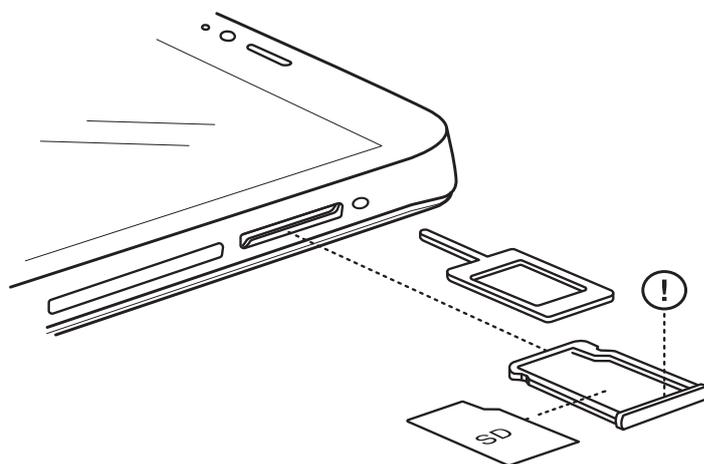
Insert the end of the SIM key into the hole of the MicroSD tray.
