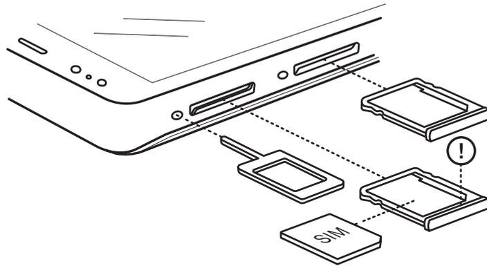
You can access the SIM trays from the exterior of the device. Do not attempt to remove the battery cover.
