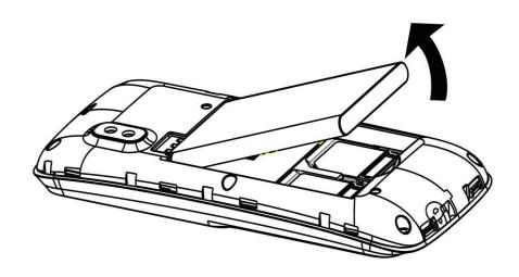
While removing battery, please bottom up the phones, remove the battery cover and pull the battery.
