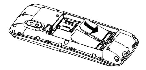
Put the SIM card into the card slot with copper sheet downward.
