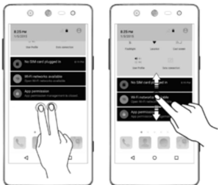
Quick Settings allow access to basic phone features such as Airplane Mode, Wi-Fi, Display Brightness, and many more.
