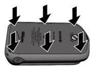
5. Using a coin, turn the battery cover screw clockwise until the cover locks.
