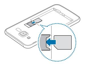
► Dual SIM models: Insert the SIM or USIM card with the gold-coloured contacts facing downwards.
