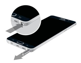
**Caution**: When you insert the S Pen into the slot, insert the S Pen's nib first. Failure to do so can cause the S Pen to become stuck. Forcefully detaching the S Pen from the slot may cause damage to the S Pen and your device.
