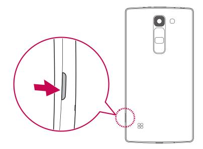
2 Slide the SIM card into the SIM card slot as shown in the figure. Make sure the gold contact area on the card is facing downward.
