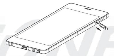
2. Insert the Micro-SIM card correctly in Micro-SIM tray.
