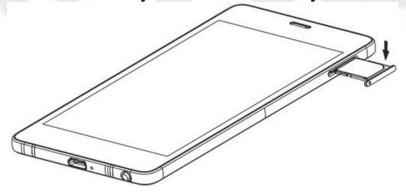
3. Push the Micro-SIM tray into the card slot.
