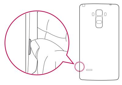
2 Slide the SIM card into the SIM card slot as shown in the figure. Make sure the gold contact area on the card is facing downward.
