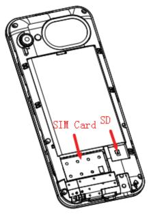
**Warning:** Be sure to remove the battery before taking inserting SIM or memory card. There is absolutely prohibited in the case of an external power supply connected during insertion or removing the SIM, or SIM card and mobile phone may be damaged.
