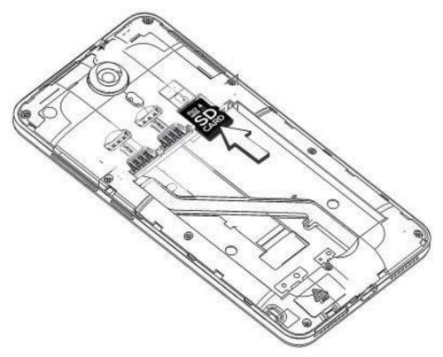
3. After inserting the memory card, place the back cover and battery of the mobile phone.
