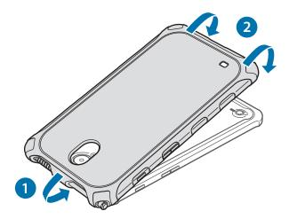
To remove the protective case from the device, twist the top edge of the case until the device protrudes from it. Then remove the device from the case.
