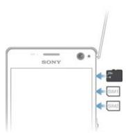
Don't confuse the nano SIM card slot with the memory card slot. Inserting a card in the wrong slot could damage both the card and your device.
